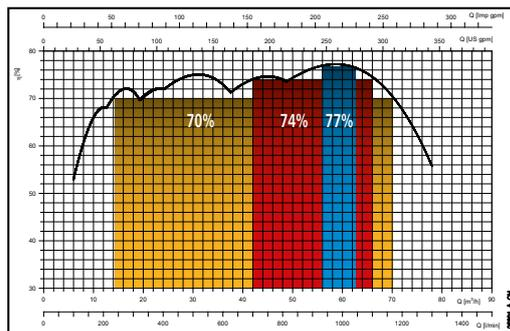
All the new Z6 series pumps offer a superior efficiency and therefore all points selected between 14 m<sup>3</sup>/h and 70 m<sup>3</sup>/h have always efficiency equal to or higher than 70% with a max efficiency of 77% within the overall Z6 range.
